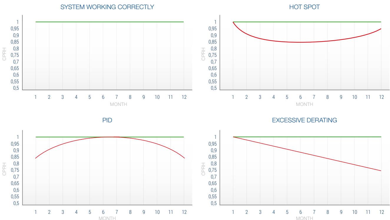
Figure 1. Negative Pattern Recognition The first box shows the normal trend in hourly corrected performance ratio (CPRh); the following boxes, in clockwise order, show patterns that identify problems relating to hot spots, PID and excessive derating.
